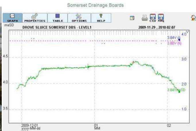
Remote telemetry provides a continuous record of water levels from key locations on Southlake
