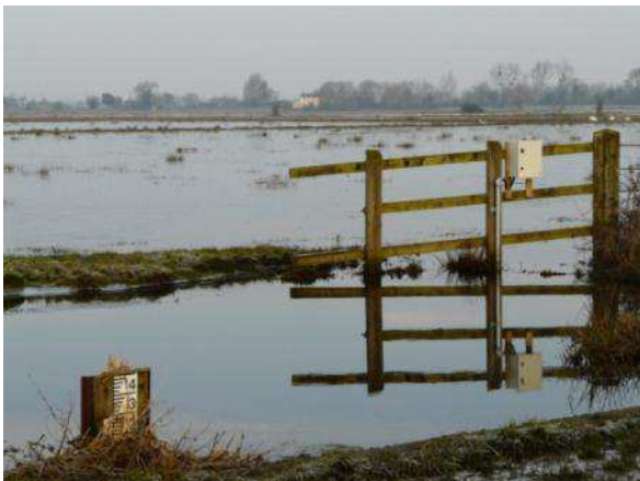
Remote telemetry provides a continuous record of water levels from key locations on Southlake
